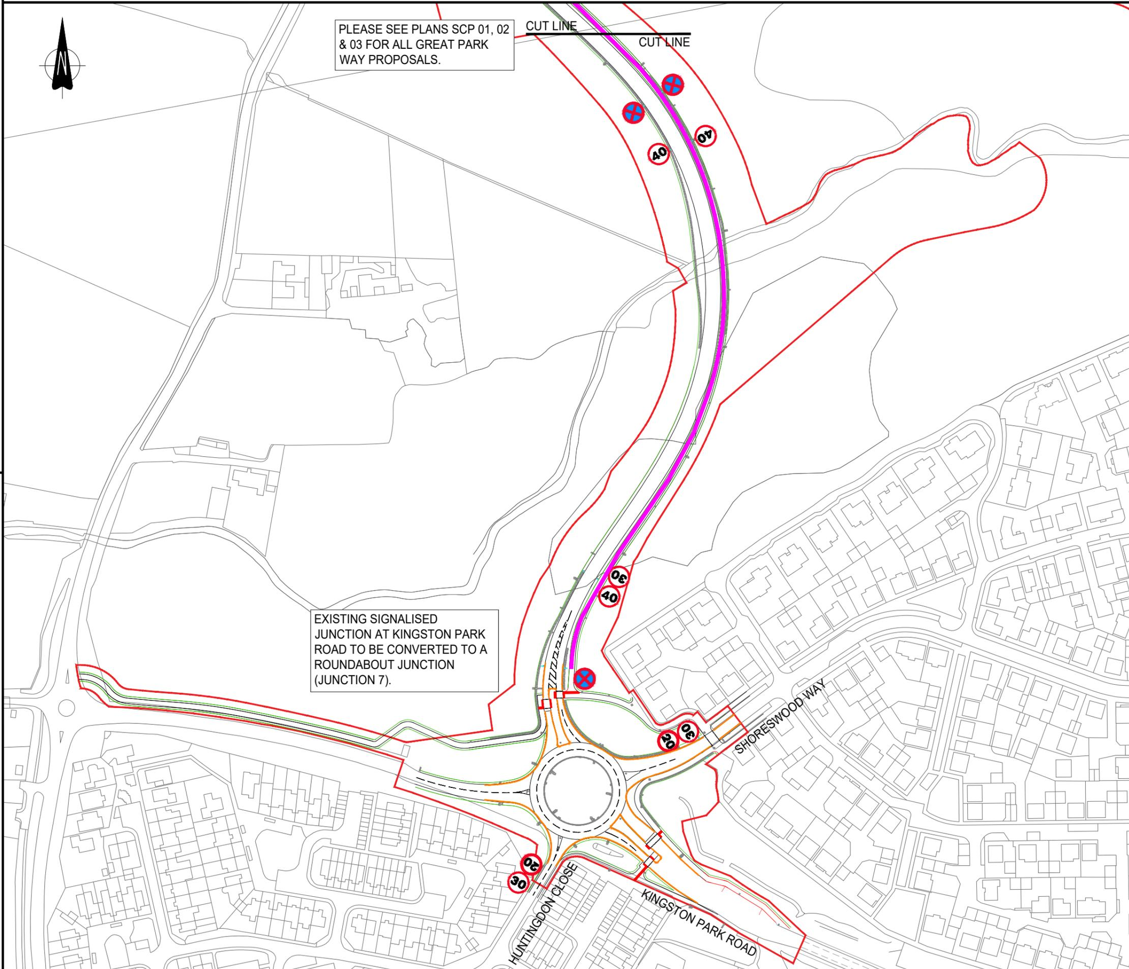
EXISTING SIGNALISED JUNCTION AT KINGSTON PARK ROAD TO BE CONVERTED TO A ROUNDABOUT JUNCTION (JUNCTION 7).
